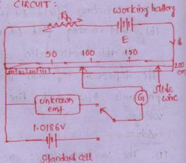
potentiometer is required to be standardized before making measurement by a std. cell.
