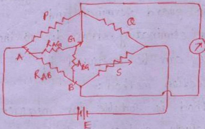
If it is measured with wheatstone then it will give  $5M\Omega$ . but with guard  $\rightarrow 10M\Omega$ .
