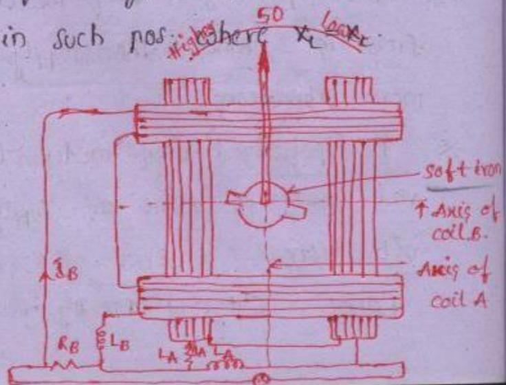
The meter consists of 2 coils mounted  $\perp^{\text{er}}$  to each other. Each coil is divided into 2 parts. coil A is connected in series with resistance  $R_A$  and whole setup placed across  $L_A$ .
