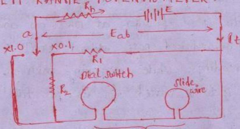
This P.M is useful to select two ranges without disturbing the calibrations.
