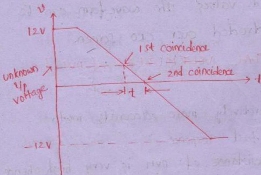
Operating principle is to measure the time that a linear ramp takes time to change from unknown i/p volt. level to ground
