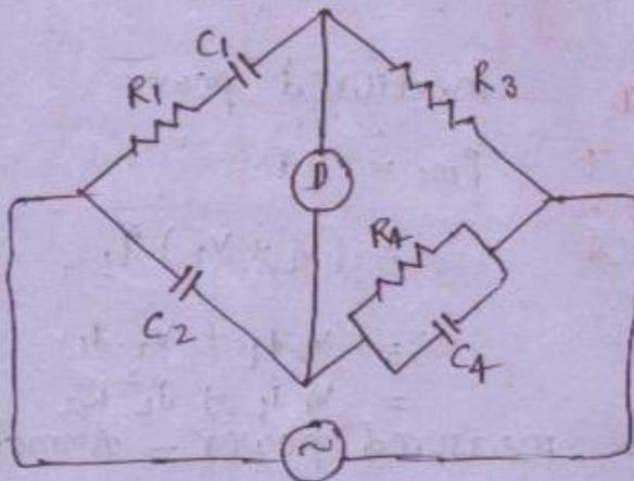
$$C_1 = \frac{R_4}{R_3} \times C_2$$
