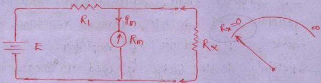
If  $R_x = 0$ , the current passing through the meter is zero, hence the pointer occupies left most position on the scale.
