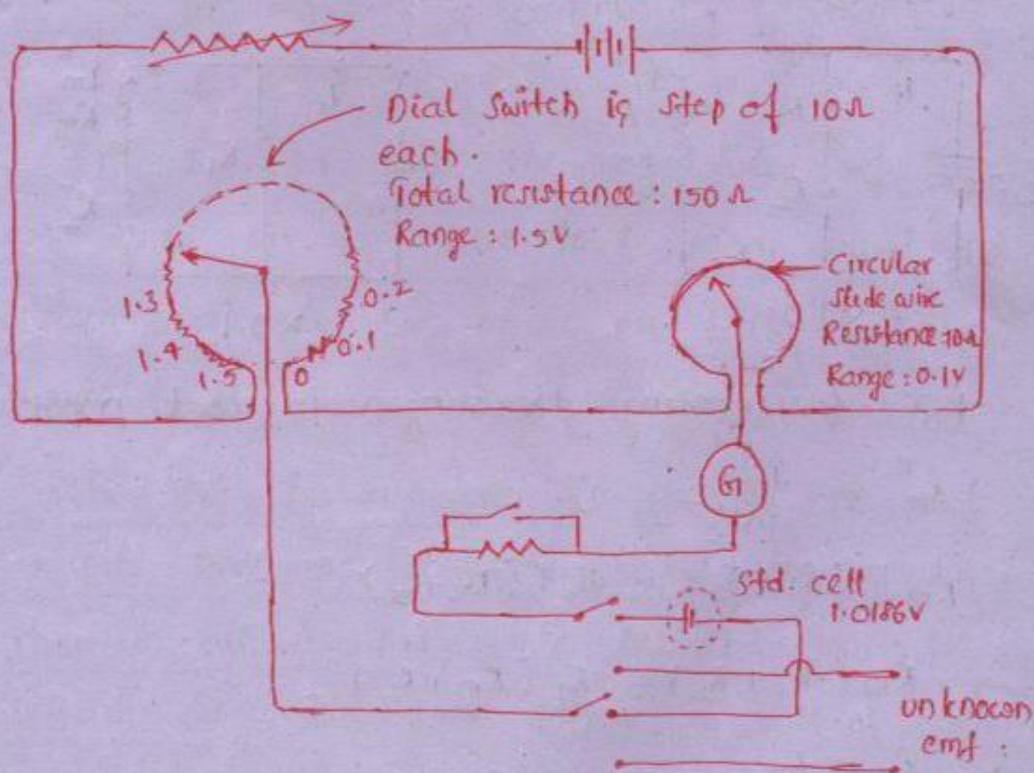
straight slide wire in basic potentiometer is replaced by dial switch & circular slide wire.
