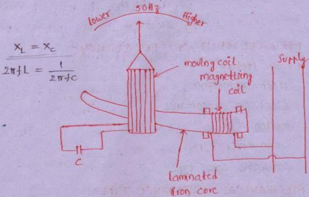
Operating principle based on electrical resonance.
